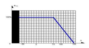
dissipation applies only if the permitted film temperature is not exceeded. These resistors do not feature a limited lifetime when operated within the permissible limits. However, resistance value drift increasing over operating time may result in exceeding a limit acceptable to the specific application, thereby establishing a functional lifetime.
